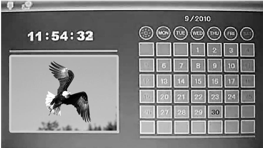
Select **Calendar** from the main menu, press **OK** to enter, the calendar is displayed and slideshow will play automatically in the left window. Adjust the date by using ◀▶.
