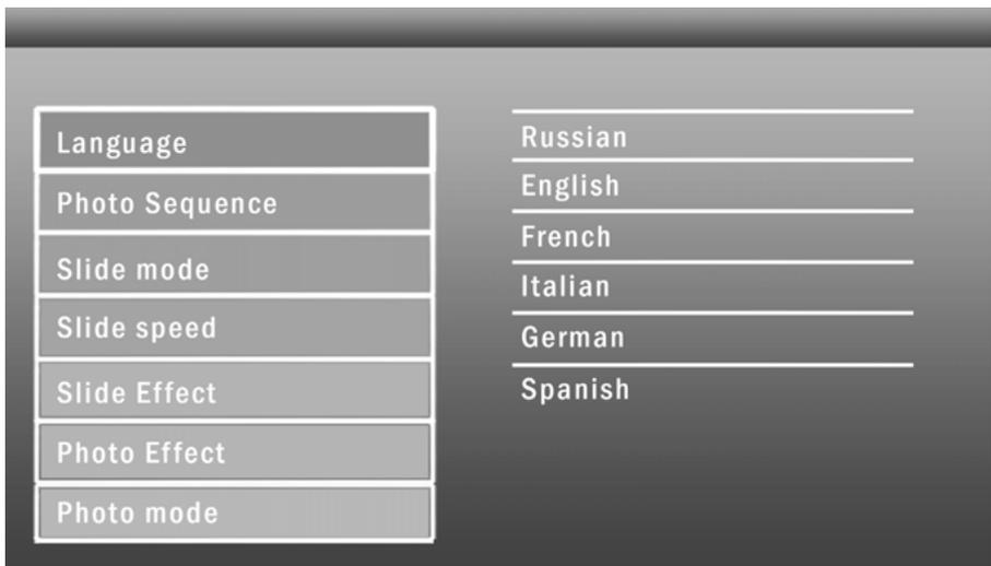
Press **Setup** from the main menu, then press **OK** to access to Set-up interface. Use ◀▶ to select the item you want to set up. Press **OK** to show the sub menu, select with ◀▶, then press **OK** to confirm.
