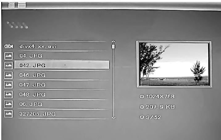
Press **EXIT** to choose «**MEMORY CARD**» or «**USB**» in the Card choose interface. Select **File**, then press **OK** to access to file interface. You can browse all the files in the memory card in this mode, and press **MENU** to delete file in built-in memory or external devices.
