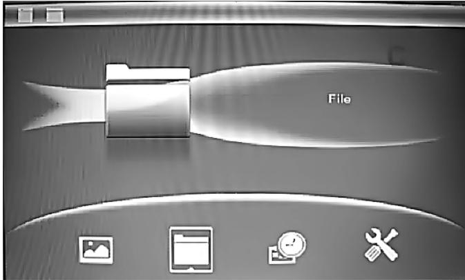
It supports SD/MMC/SDHC and USB 2.0. After inserting a card or USB device, slideshow will play automatically, then press **Exit** twice to access to **Main menu**, you can view **Photo**, **File**, **Calendar** and **Set-up** icon on this interface. Press **OK** to confirm your selection.
