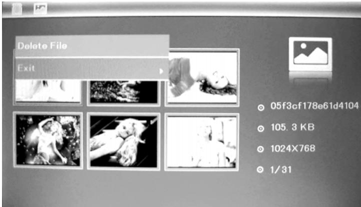
Delete pictures in built-in memory or memory card: In six-picture mode, use ◀▶ to select the picture you want to delete in the built-in memory or card device, then press **MENU** to enter delete interface, press **OK** to confirm.
